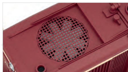
Cover over the separately attached fan wheel implemented as a delicate etched part
