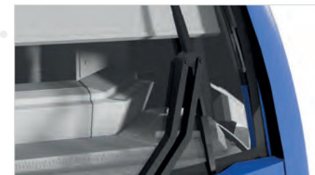
Front panel, windscreen wipers and sun blind attached separately
