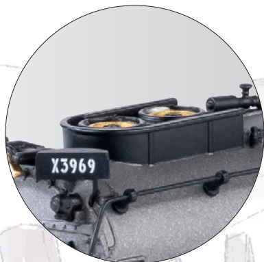
Steam exhaust via the compound smokestack
