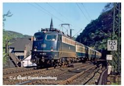
**Prototype**: German Federal Railroad (DB) standard design electric locomotive, road number 110 318-3. Nicknamed "Bügelfalte" / "Pants Crease". Cobalt blue basic paint scheme. Version with double lamps, plastic rain gutters above the end windows, and cab doors, "continuous" ventilation band consisting of 7 "Klatte Ventilation Grills long", and end grab irons. Without skirting and without buffer cladding. The locomotive looks as it did around 1983.
