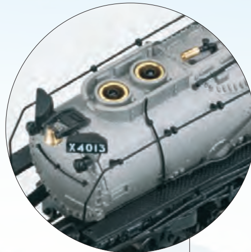
Prototypical smoke exhaust using two smoke stacks
