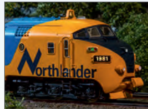
Classification Lights – they are designated as limit lights and give information about the status of the train
