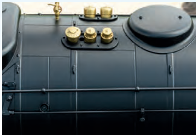
The safety vents on the model were made of brass to conform to the prototype
