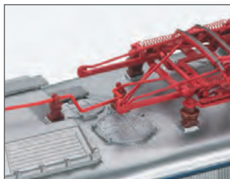
The conductors on the roof insulators also run prototypically
