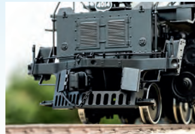
The front coupler is hidden in a refined manner behind two hatches
