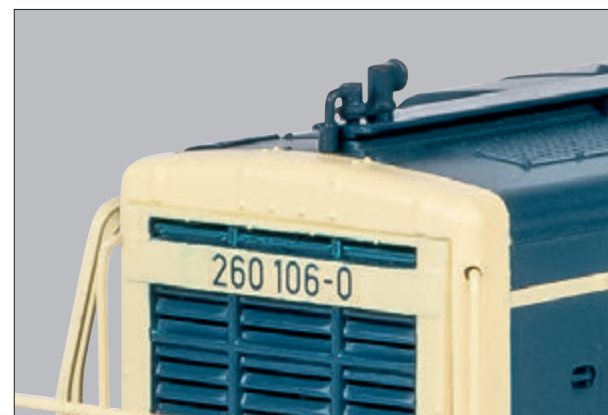
Ventilation grilles on the end and modern coolant indicator with display instrument on the nose section
