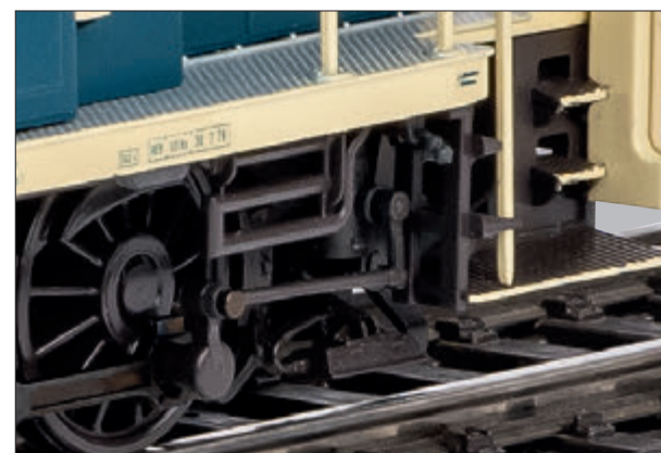
With inductive magnets on both sides and an operational motor for the wheel flange lubrication
