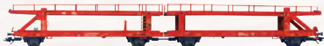
47180 Type Laaeks 553.1 Double Auto Transport Car – Use the DC wheelset E700580 for the exchange
